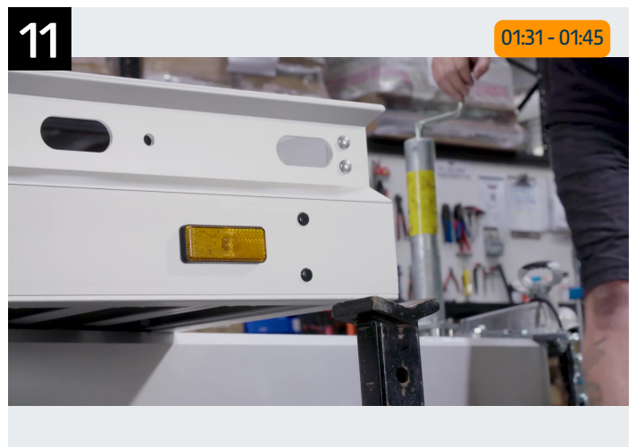
Place jack stands under the trailer and lower it onto them.
